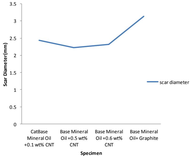
**Figure 2.** Scar diameters on balls.
