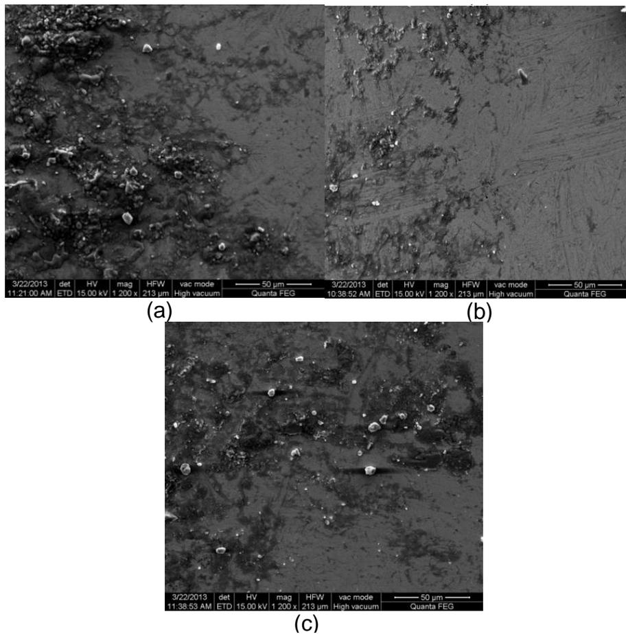
**Figure 3.** SEM image of metal ball used in four ball tester for pass load of (a) mineral oil (b) Mineral oil +0.5% wt CNT (c) Mineral oil + 0.5% Graphite.
