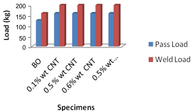
**Figure 1.** Pass Load and Weld Load values from the Four Ball Test.**Table 3.** Scar diameters of different specimens.
